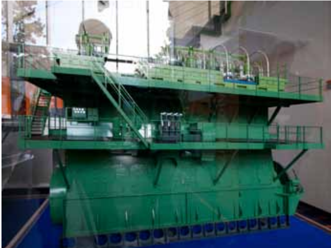
Wärtsilä 8RT – flex96c – Power: 45.760 kW; Length: 17233 mm; Speed: 102rpm; Width: 4480 mm; Weight: 1470 tons; Height: 13519 mm
